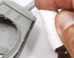
Once the pieces are joined, deposit the Activator on the cyanoacrylate, which will be completely dry in 2-3 seconds, creating a strong and durable bond.
