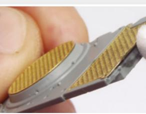
**3, 4.** Then wipe the surface clean with a cloth or cotton swab. If necessary, the process can be repeated until the cyanoacrylate residue is completely removed.
