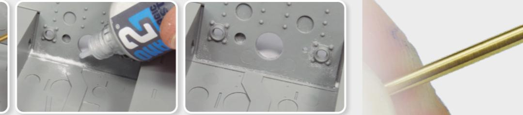
You can deposit it directly from the can onto the cyanoacrylate application or mix it with the Slow Dry Cyanoacrylates before applying it, as if it were putty.
